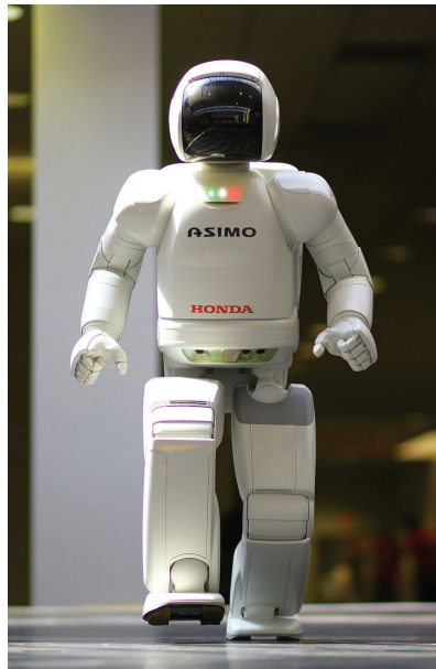
Honda keeps improving Asimo, acronym for Advanced Step in Innovative Mobility, so this robot can now walk up and down stairs, run and even play soccer. Asimo's hand and finger dexterity along with the robot's intellect are also improving. Future uses for Asimo include being an alert never-sleeping 24-hour medical attendant, becoming a space traveler and serving in businesses ranging from banks to restaurants.
