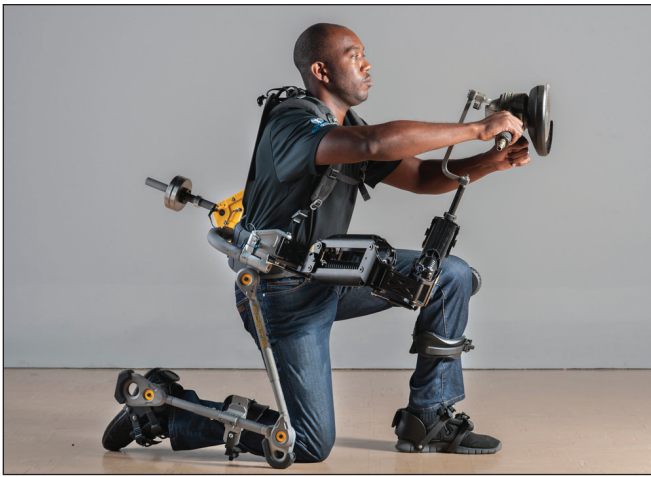
Lockheed Martin has created the FORTIS exoskeleton which can add strength to the human body and boost worker productivity up to 27 times the normal rate. Factory worker applications and military uses are being studied.
