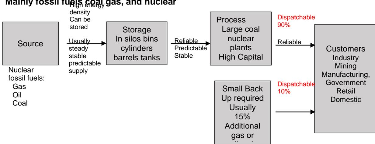
**Figure 53: System for dispatchable electricity technologies**
