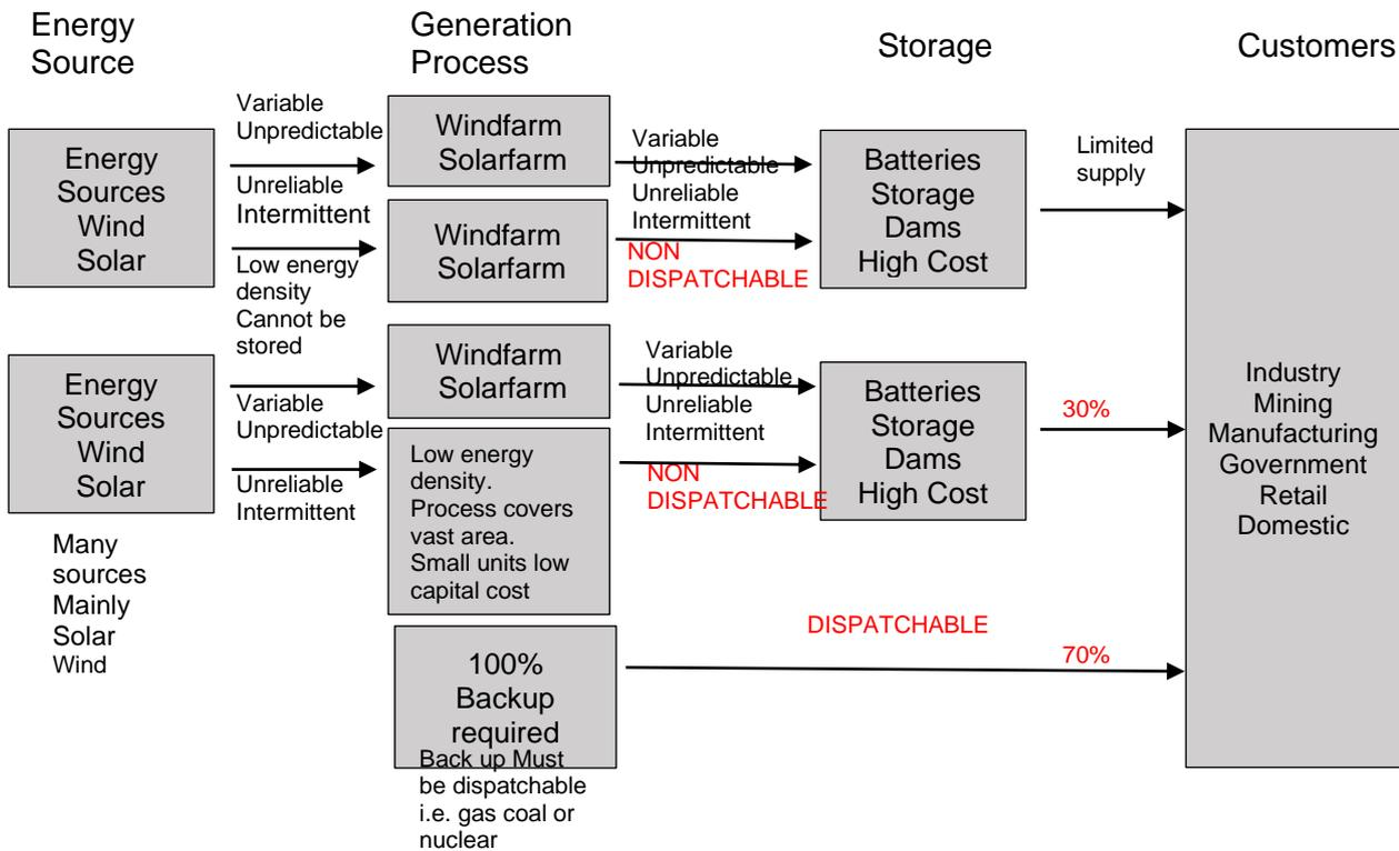
**Figure 52: System for non-dispatchable technologies**
